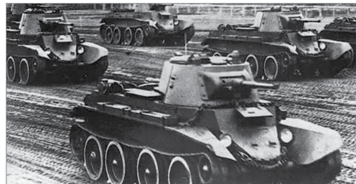
A unit of BT-7s meaning Bystrokhodny (fast-moving) tank, i.e. a cavalry tank. Their 44.7 mph top speed made them superbly mobile and their
